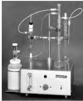
Model CM5020 Acidification Module, c. 1975 - The Model CM5020 has a stainless-steel body and "cigarette lighter" style heater. CM5020 model is obsolete.
